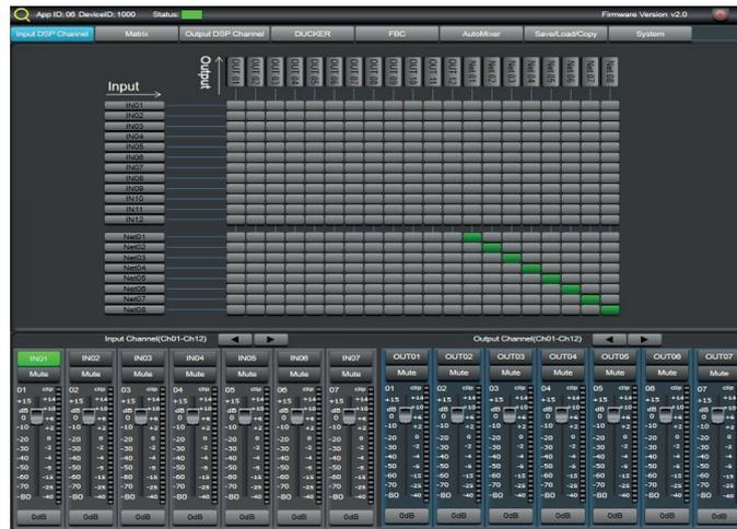
When we want to share an analogue input of an matrix on the NET channels (to be visible and selectable as an audio source by the other matrixes in the installation), we must select the analogue input we want (IN01 to IN12), mark it on the channel (NET01 to NET 08) that we want and unmark it from the diagonal NET, as follows:
